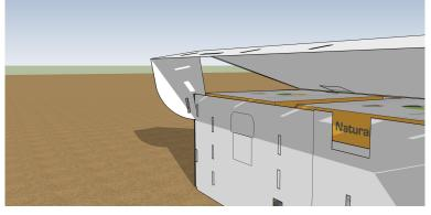
Secure the awning with the help of the two latches at the edges of the hive.
