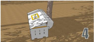
In order to secure the triple in place, it is recommended to tie it to a very stable (rod or trunk) with a string or a zip tie.
